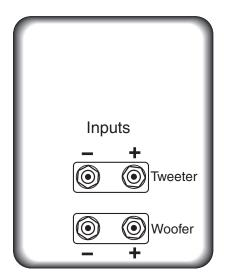
A speaker which can be biamped or biwired will have two sets of binding posts. Sometimes these posts are joined with bridge clips for normal operation.
